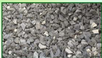
PVC Pipe Regrind
